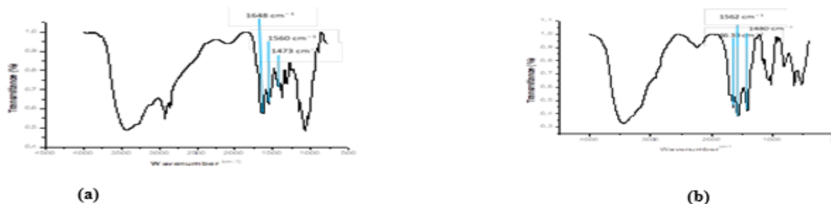
Figure 4. Infrared absorption spectra of the microbiological polymers obtained from Rhizopus arrhizus biomass as: (a) chitin and (b) chitosan.
